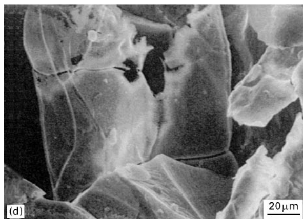
Figure 16(a-n) Scanning electron microscopy photographs of 316 Ti steel corroded in the presence of 0.02 \text{ mol dm}^{-3} \text{ Cl}^- in ^2\text{H}_2\text{O} at 1.5 V/SCE.
